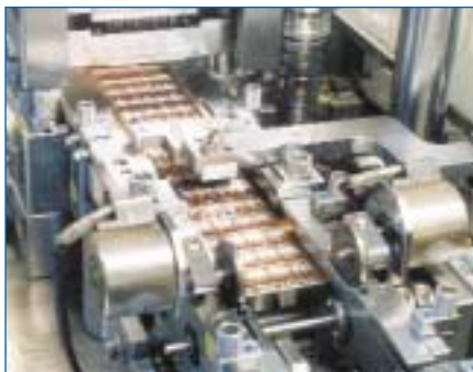
Figure 6. Photo of a CM-MS five-stage singulation system with a leadframe strip
