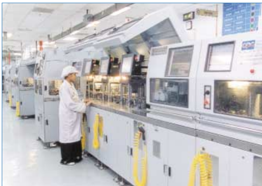
This is the singulation station of an in-line CM-MS system. The system measures 19 meters (62 feet) in length.
