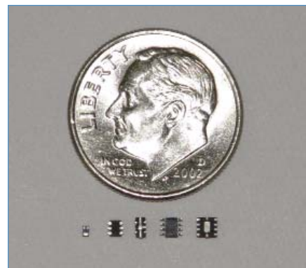
Figure 1. Left to right is a bottom view of a 3-lead SOT-883 (Mini-MLP), 6-lead SOT-666, 5-lead 2x1mm MLP, 8-lead SC70, and an 8-lead 2x2mm MLP.
