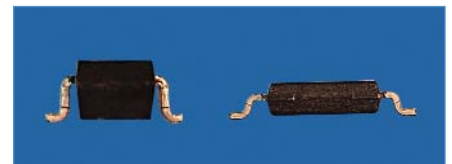
Figure 4. This figure compares an end view of a SOT23 micro-package with an MSOP. (not to scale)
